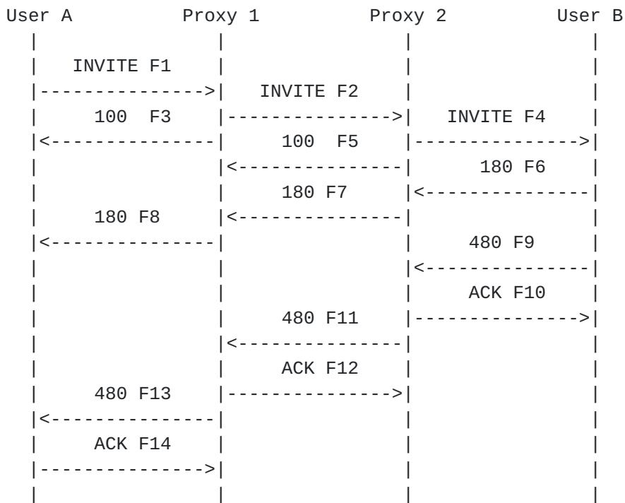
In this scenario, User B initially sends a 180 Ringing response to User A, indicating that alerting is taking place. However, then a 480 Unavailable is then sent to User A. This response is acknowledged then proxied back to User A.
