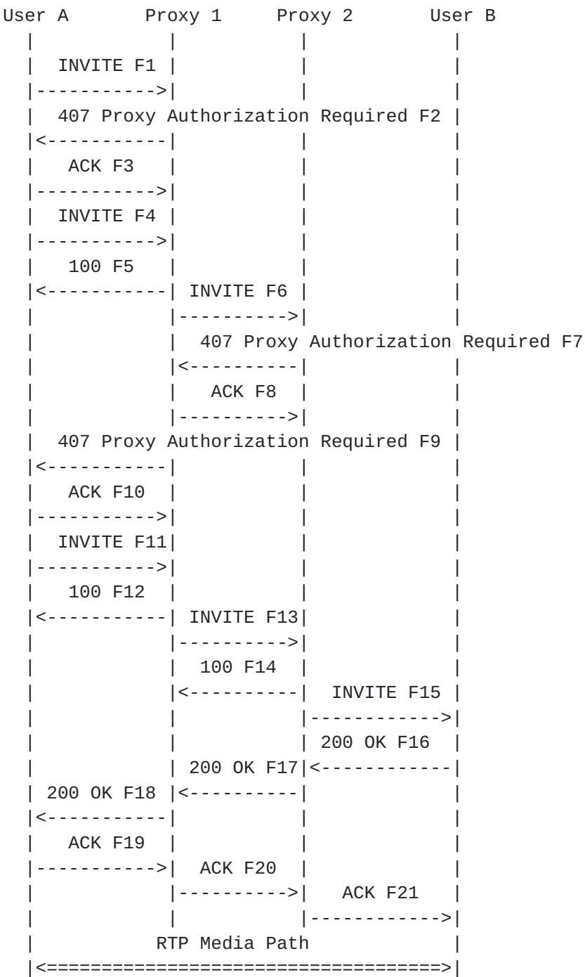
In this scenario, User A completes a call to User B using two proxies Proxy 1 and Proxy 2. User A has valid credentials in both domains. Since the initial INVITE (F1) does not contain the Authorization credentials Proxy 1 requires, so a 407 Proxy Authorization response is sent containing the challenge information. A new INVITE (F4) is then sent containing the correct credentials and the call proceeds after Proxy 2 challenges and receives valid
