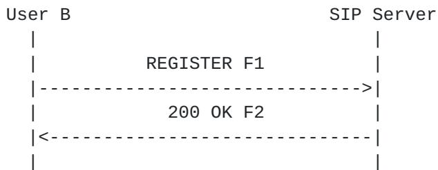
User B sends a register request to the Proxy Server containing no Contact headers, indicating the user wishes to query the server for the user's current contact list. Since the user already has authenticated with the server, the user supplies authentication credentials with the request and is not challenged by the server. The SIP server validates the user's credentials. The server returns a response (200 OK) which includes the user's current registration list in Contact headers.
