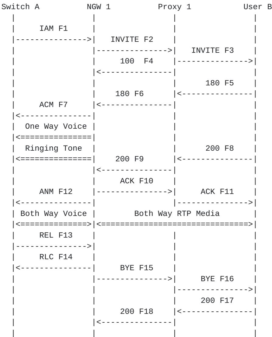
In this scenario, User A from the PSTN calls User B through a Network Gateway NGW1 and Proxy Server Proxy 1. When User B answers the call the media path is setup end-to-end. The call terminates when User A hangs up the call, with User A's telephone switch sending an ISUP RELEase message which is mapped to a BYE by NGW 1.
