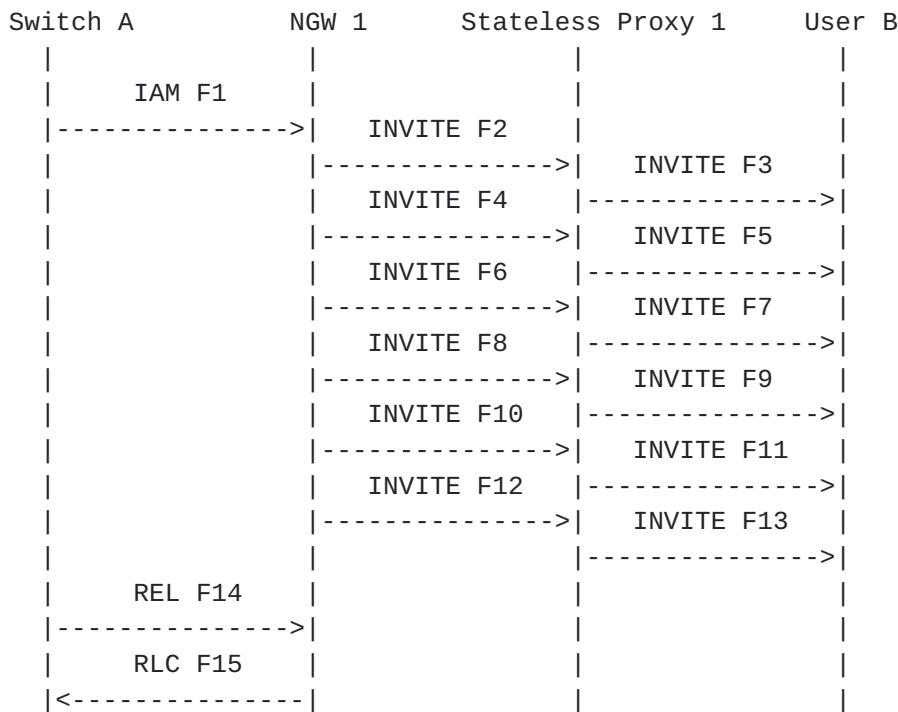
In this scenario, User A calls User B through NGW 1 and Proxy 1. Since Proxy 1 is stateless (it does not send a 100 Trying response), NGW 1 re-sends the INVITE message after the expiration of SIP timer T1. User B does not respond with 180 Ringing. User A's network disconnects the call with a release REL (CauseCode=102 Timeout).
