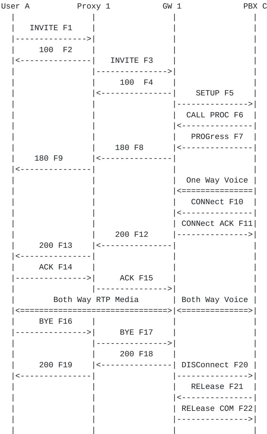
User A is a SIP device while User C is connected via a Gateway (GW 1) to a PBX. The PBX connection is via a ISDN trunk group. User A dials User C's telephone number (918-555-3333) which is globalized and put into a SIP URI.
