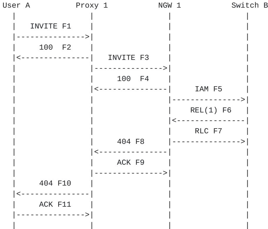
User A calls PSTN User B through a Proxy Server Proxy 1 and a Network Gateway NGW 1. The call is rejected by the PSTN with a ANSI ISUP Release message REL containing a specific Cause code. This cause value (1) is mapped by the Gateway to a SIP 404 Address Incomplete response which is proxied back to User A. For more details of ISUP cause value to SIP responses refer to [[SIP-ISUP](#)].
