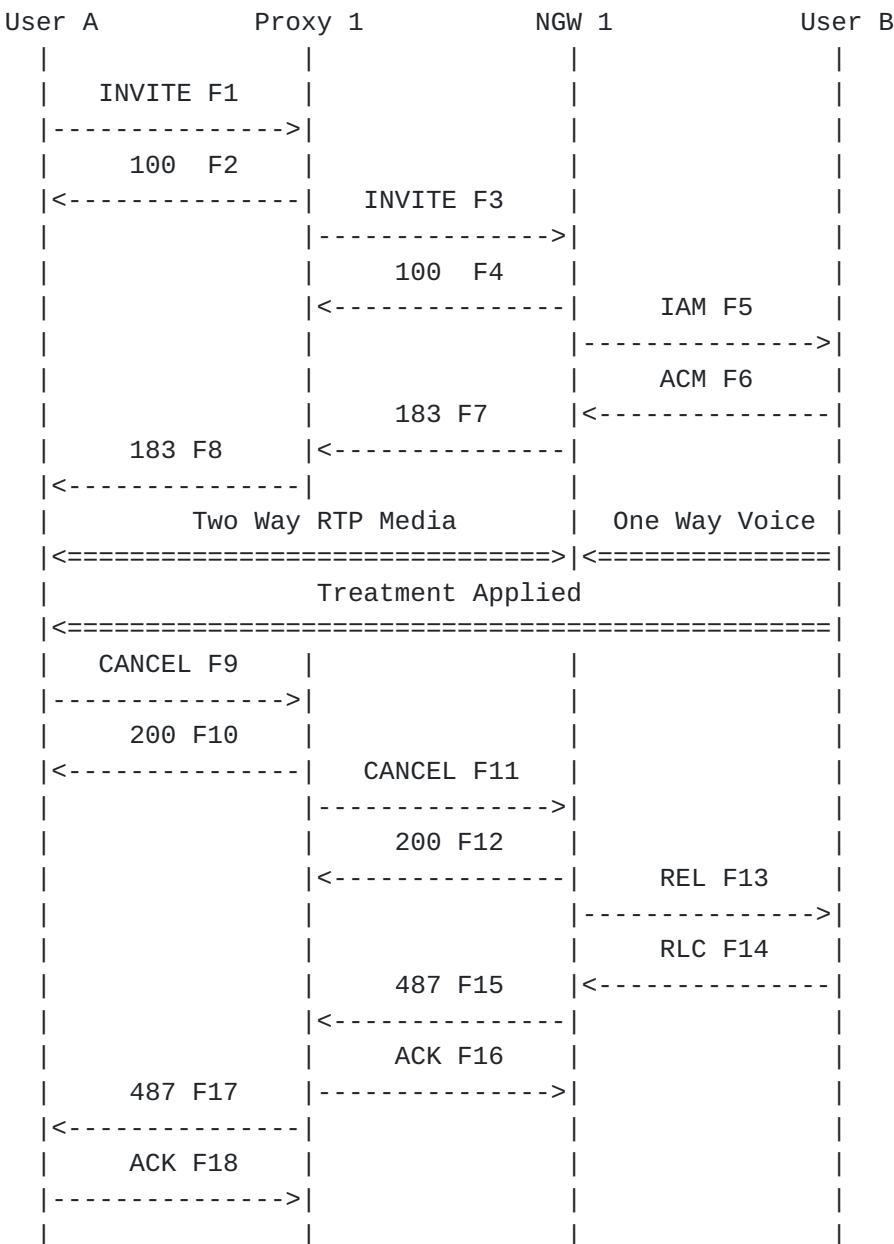
User A calls User B in the PSTN through a proxy server Proxy 1 and a Network Gateway NGW 1. The call is rejected by the PSTN with an in-band treatment (tone or recording) played. User A hears the treatment and then hangs up, which results in a CANCEL (F9) being sent to terminate the call. (A BYE is not sent since no final response was ever received by User A.)
