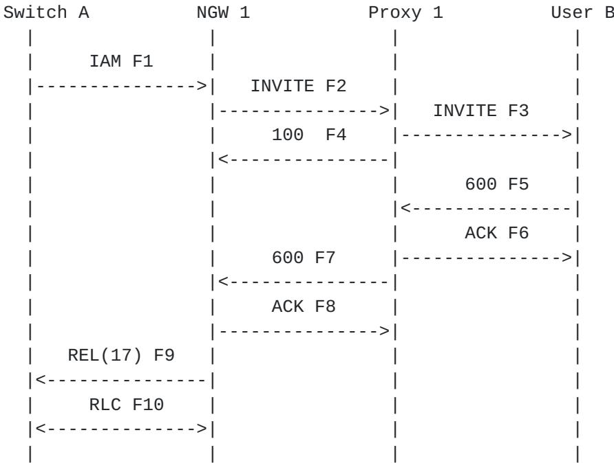
In this scenario, User A calls User B through Network Gateway NGW 1 and Proxy 1. The call is routed to User B by Proxy 1. The call is rejected by User B who sends a 600 Busy Everywhere response. The Gateway sends a REL message containing a specific Cause value mapped by the gateway based on the SIP error.
