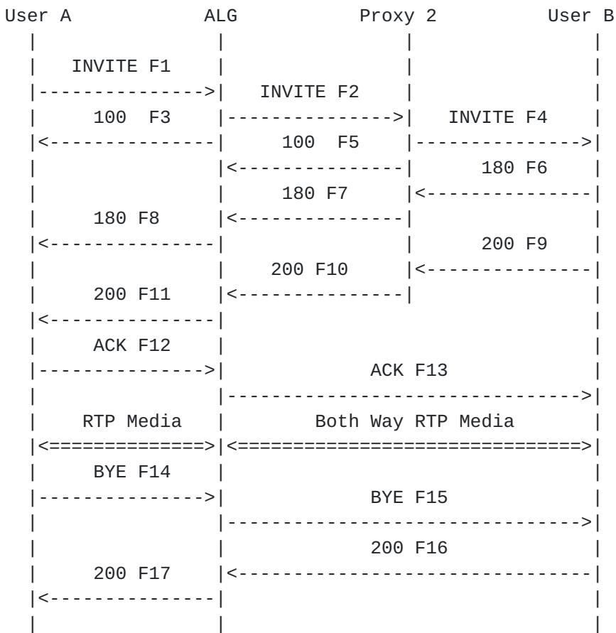
User A completes a call to User B through a ALG (Application Layer Gateway) and a SIP Proxy. The routing through the ALG is accomplished using a pre-loaded Route header in the INVITE F1. Note that the media stream setup is not end-to-end - the ALG terminates both media streams and bridges them. This is done by the ALG modifying the SDP in the INVITE (F1) and 200 OK (F10) messages, and possibly any 18x or ACK messages containing SDP.
