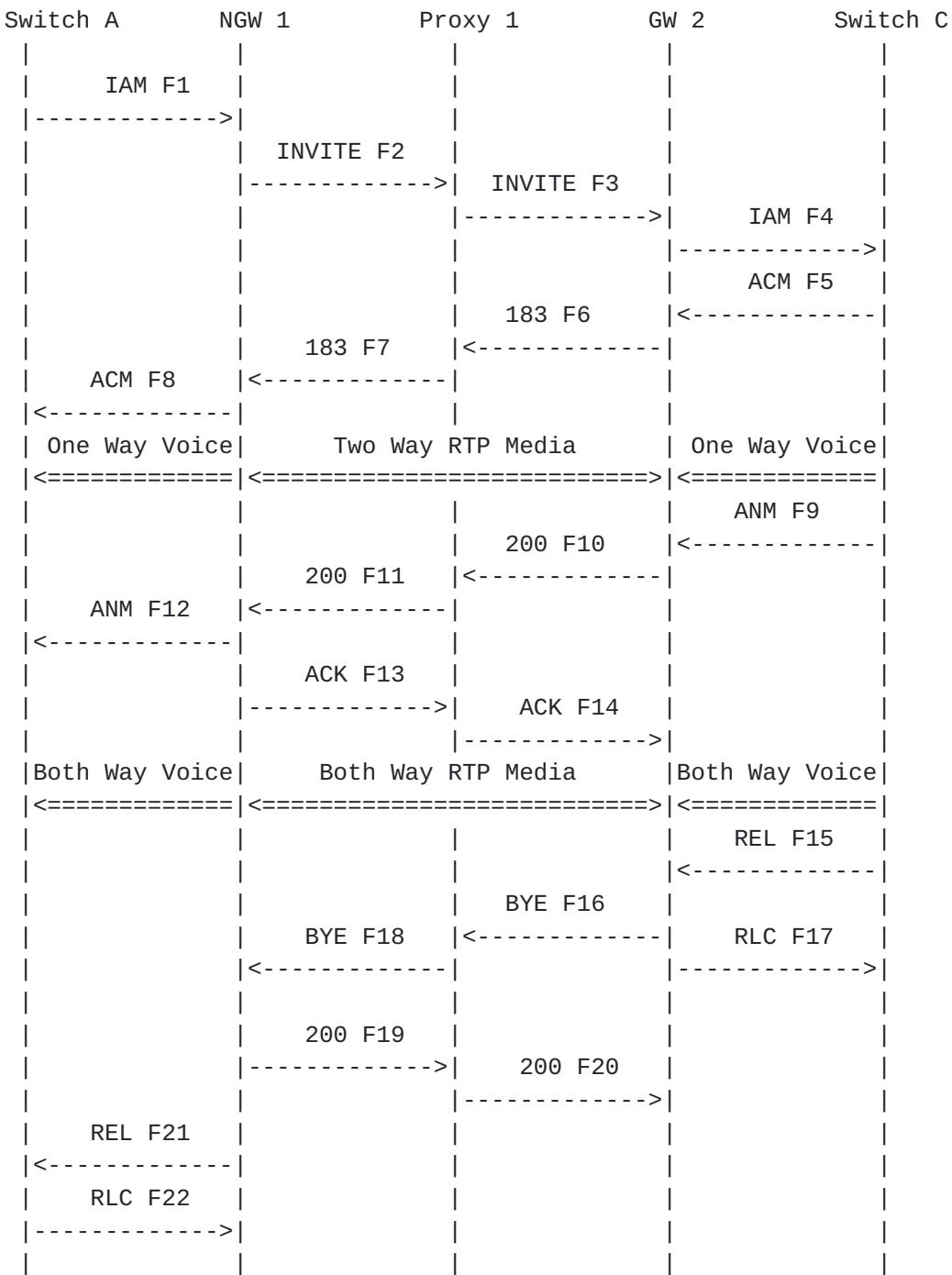
In this scenario, User A in the PSTN calls User C who is an extension on a PBX. User A's telephone switch signals via SS7 to the Network Gateway NGW 1, while User C's PBX signals via SS7 with the Gateway GW 2. The CdPN and CgPN are mapped by GW1 into SIP URIs and placed in the To and From headers. Proxy 1 looks up the dialed digits in the Request-URI and maps the digits to the PBX extension of
