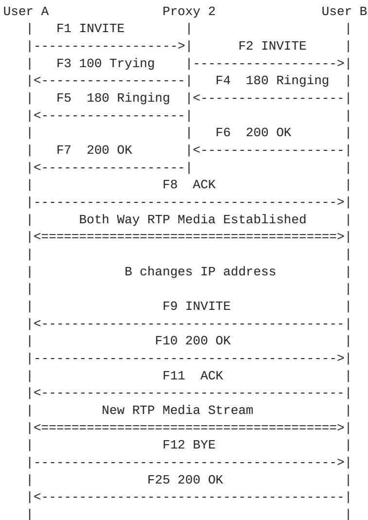
This example shows a session in which the media is changes midway through the session. When User B's IP address changes during the session, User B sends a re-INVITE containing a new Contact and SDP (version number incremented) information to A. In this flow, the proxy does not Record-Route so is not in the SIP messaging path after the initial exchange.
