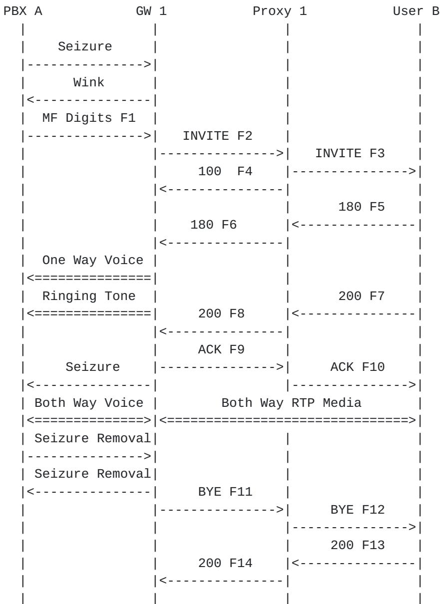
In this scenario, User A dials from PBX A to User B through GW 1 and Proxy 1. This is an example of a call that appears destined for the PSTN but instead is routed to a SIP Client.
