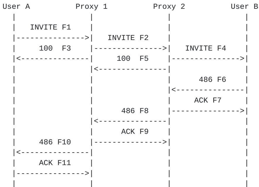
In this scenario, User B is busy and sends a 486 Busy Here response to User A's INVITE. Note that the non-2xx response is acknowledged on a hop-by-hop basis instead of end-to-end.
