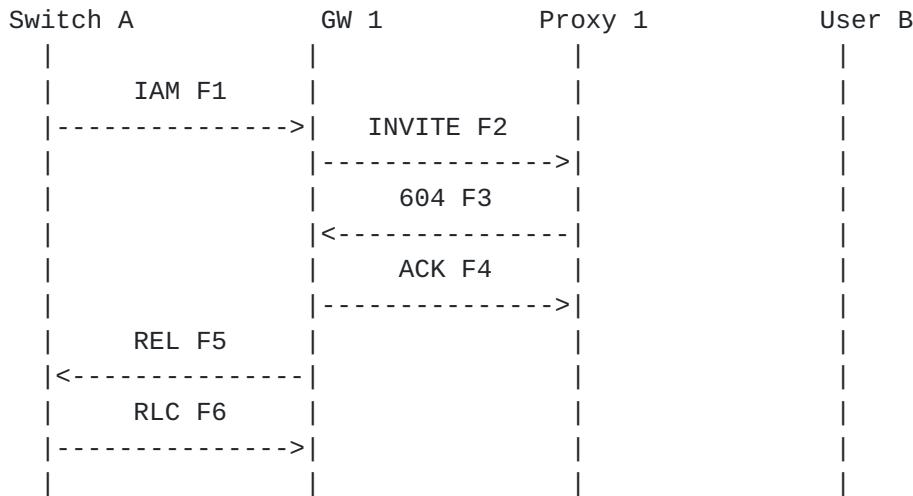
User A attempts to place a call through Gateway GW 1 and Proxy 1, which is unable to find any routing for the number. The call is rejected by Proxy 1 with a REL message containing a specific Cause value mapped by the gateway based on the SIP error.
