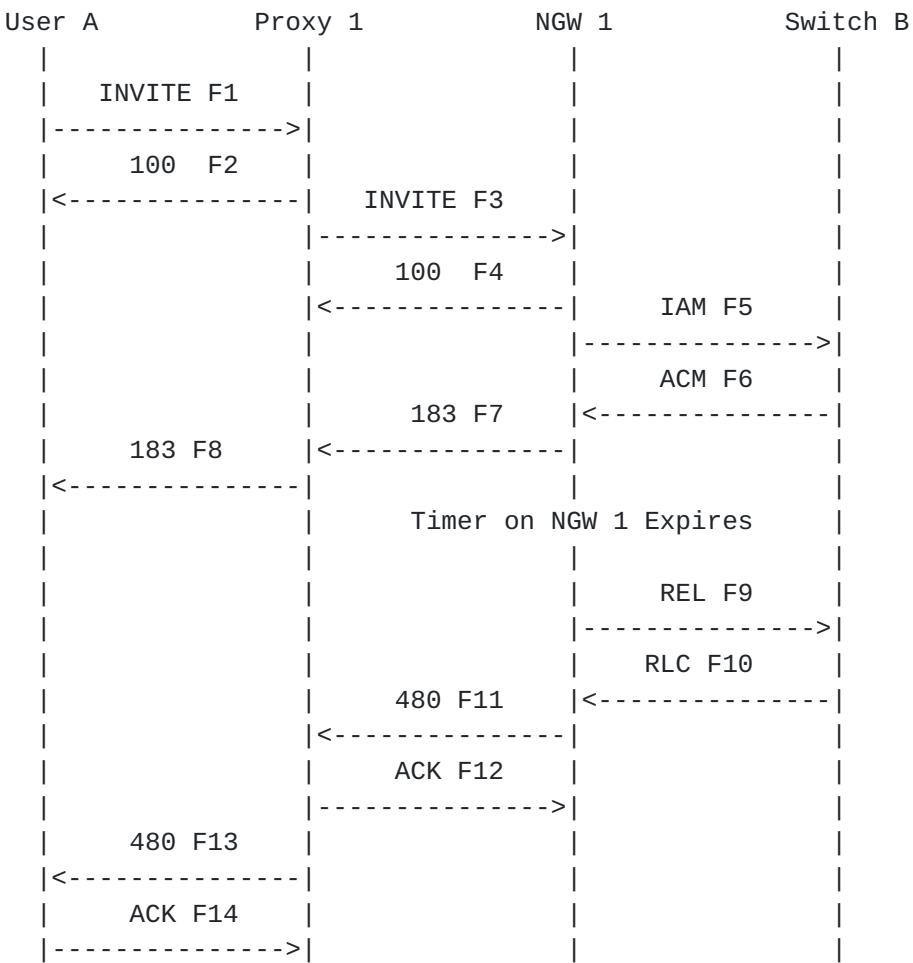
User A calls User B in the PSTN through a proxy server Proxy 1 and Network Gateway NGW 1. The call is released by the Gateway after a timer expires due to no ANswer Message (ANM) being received. The Gateway sends an ISUP Release REL message to the PSTN and a 480 Temporarily Unavailable response to User A in the SIP network.
