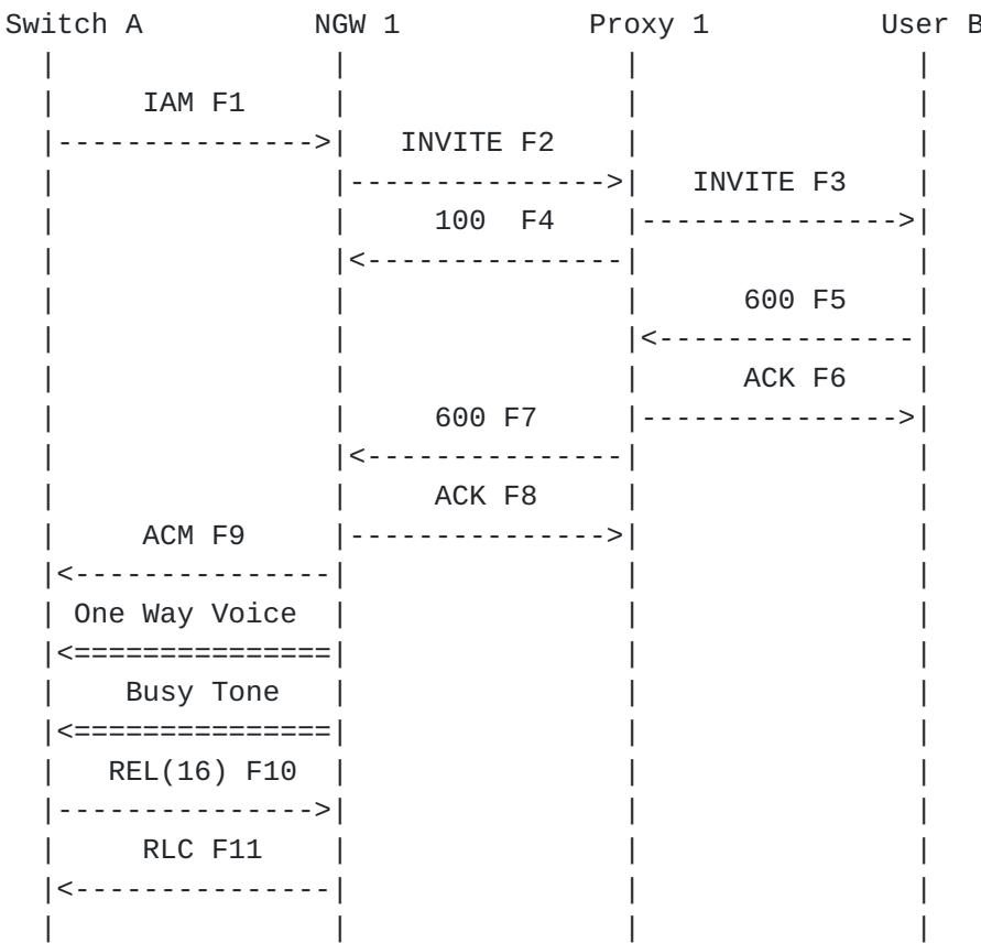
In this scenario, User A calls User B through Network Gateway NGW1 and Proxy 1. The call is routed to User B by Proxy 1. The call is rejected by the User B client. NGW 1 sets up a two way voice path to User A and plays busy tone. The caller then disconnects.
