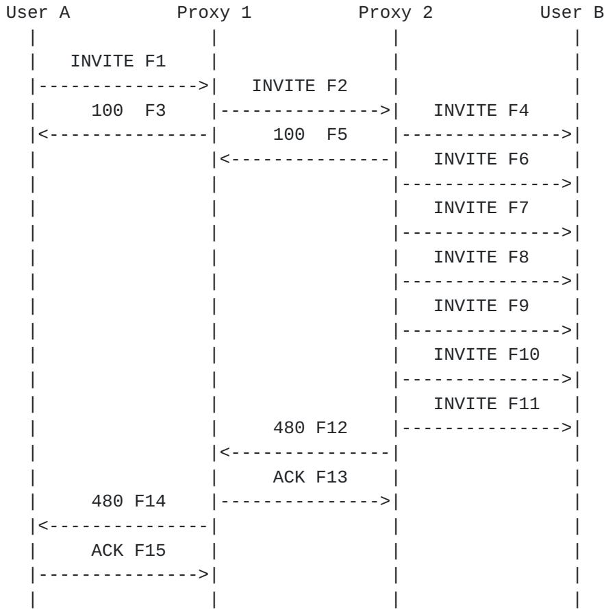
In this example, there is no response from User B to User A's INVITE messages being re-transmitted by Proxy 2. After the sixth re-transmission, Proxy 2 gives up and sends a 480 No Response to User A.
