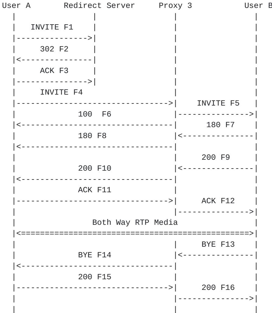
In this scenario, User A places a call to User B using first a Redirect server then a Proxy Server. The INVITE message is first sent to the Redirect Server. The Server returns a 302 Moved Temporarily response (F2) containing a Contact header with User B's current SIP address. User A then generates a new INVITE and sends to User B via the Proxy Server and the call proceeds normally. In this example, no SDP is present in the INVITE, so the SDP is carried in the ACK message.
