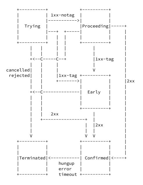
Figure 1: Dialog finite state machine
