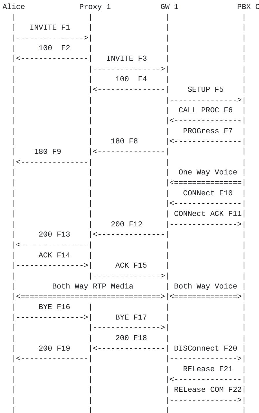
Alice is a SIP device while Carol is connected via a Gateway (GW 1) to a PBX. The PBX connection is via a ISDN trunk group. Alice dials Carol's telephone number (918-555-3333) which is globalized and put into a SIP URI.
