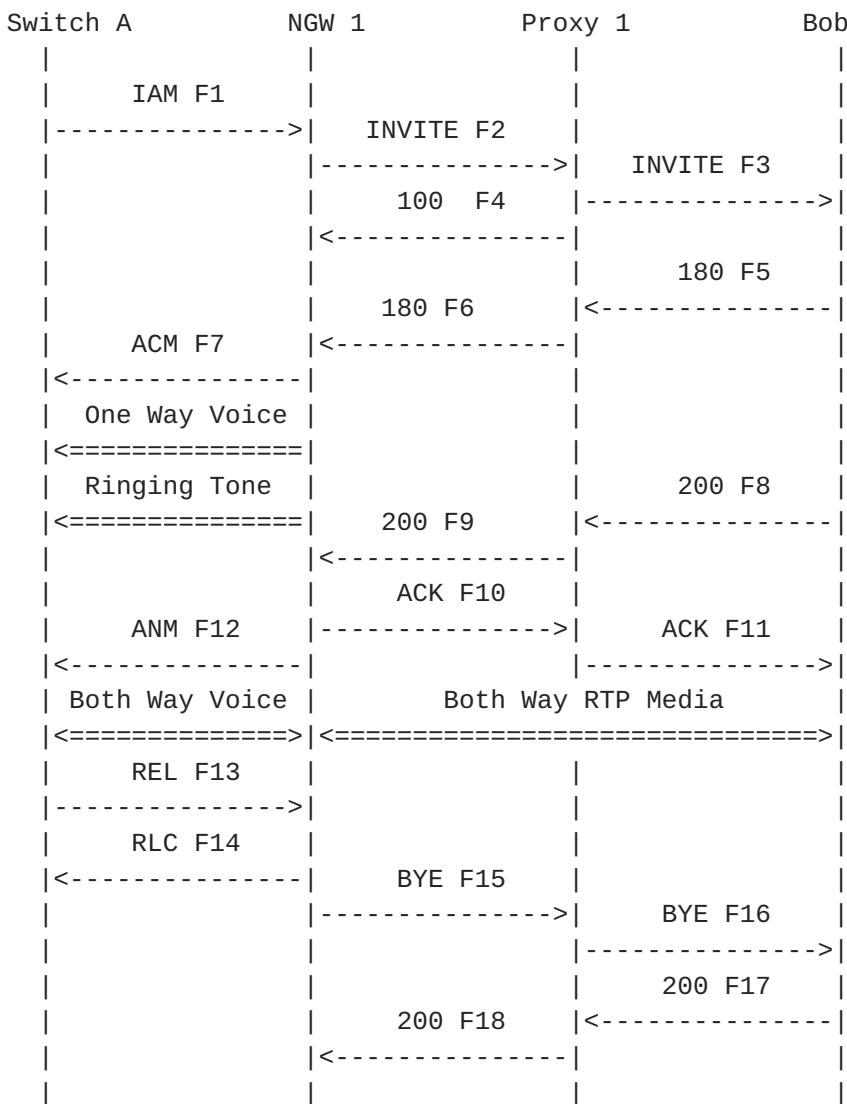
In this scenario, Alice from the PSTN calls Bob through a Network Gateway NGW1 and Proxy Server Proxy 1. When Bob answers the call the media path is setup end-to-end. The call terminates when Alice hangs up the call, with Alice's telephone switch sending an ISUP RERelease message which is mapped to a BYE by NGW 1.
