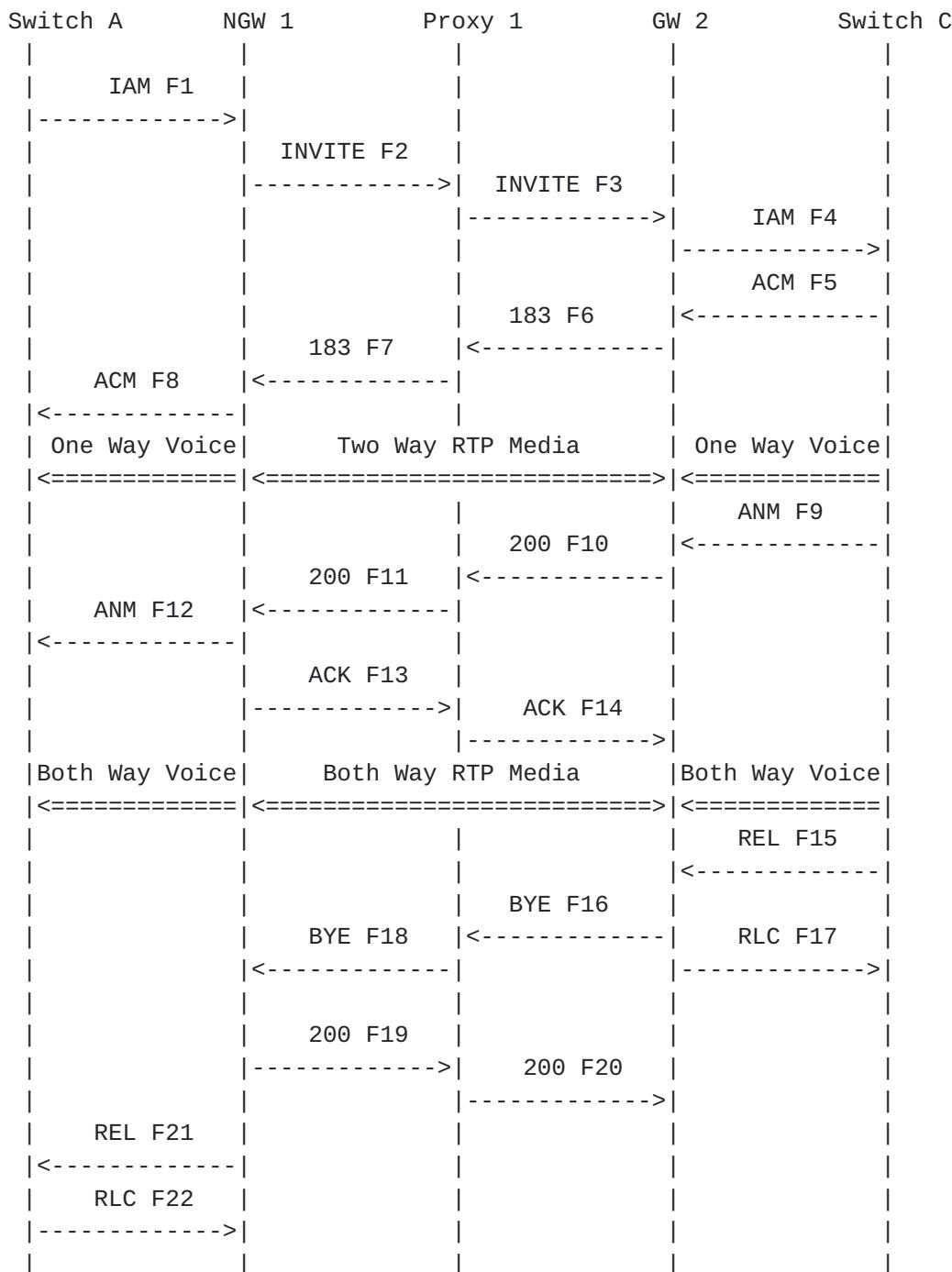
In this scenario, Alice in the PSTN calls Carol who is an extension on a PBX. Alice's telephone switch signals via SS7 to the Network Gateway NGW 1, while Carol's PBX signals via SS7 with the Gateway GW 2. The CdPN and CgPN are mapped by GW1 into SIP URIs and placed in the To and From headers. Proxy 1 looks up the dialed
