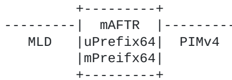
Figure 4: MLD-PIMv4 Interworking Function
