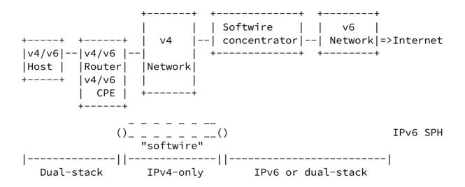
Case 3: IPv6 connectivity across an IPv4-only access network (STH). The CPE is IPv4-only. Softwire initiator is a host, which act as an IPv6 host CPE. The IPv4 traffic should not traverse the softwire.
