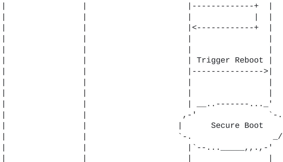
Figure 6: Second Example Flow for a Firmware Upate.
