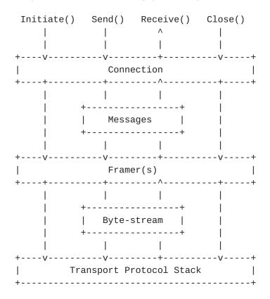
Note that while Message Framers add the most value when placed above a protocol that otherwise does not preserve message boundaries, they can also be used with datagram- or message-based protocols. In these cases, they add an additional transformation to further encode or encapsulate, and can potentially support packing multiple application-layer Messages into individual transport datagrams.
