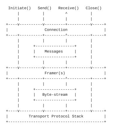
Figure 1: Protocol Stack showing a Message Framer
