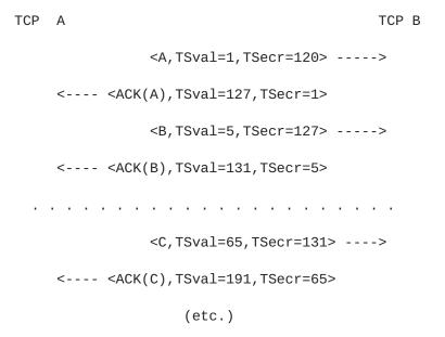
The dotted line marks a pause (60 time units long) in which A had nothing to send. Note that this pause inflates the RTT which B could infer from receiving TSecr=131 in data segment C. Thus, in one-way data flows, RTTM in the reverse direction measures a value that is inflated by gaps in sending data. However, the following rule prevents a resulting inflation of the measured RTT:
