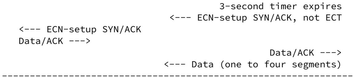
Figure 1: SYN exchange with the SYN/ACK packet dropped.
