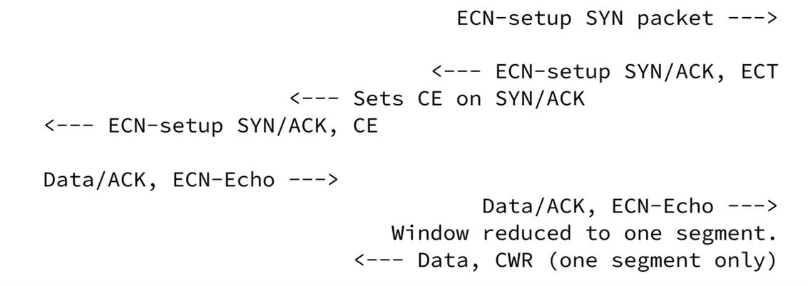
Figure 2: SYN exchange with the SYN/ACK packet marked.
