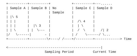
Figure 1: Example of measuring pipeACK samples
