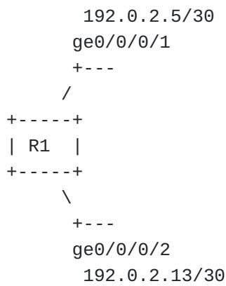
Figure 6: Example of network configuration.
