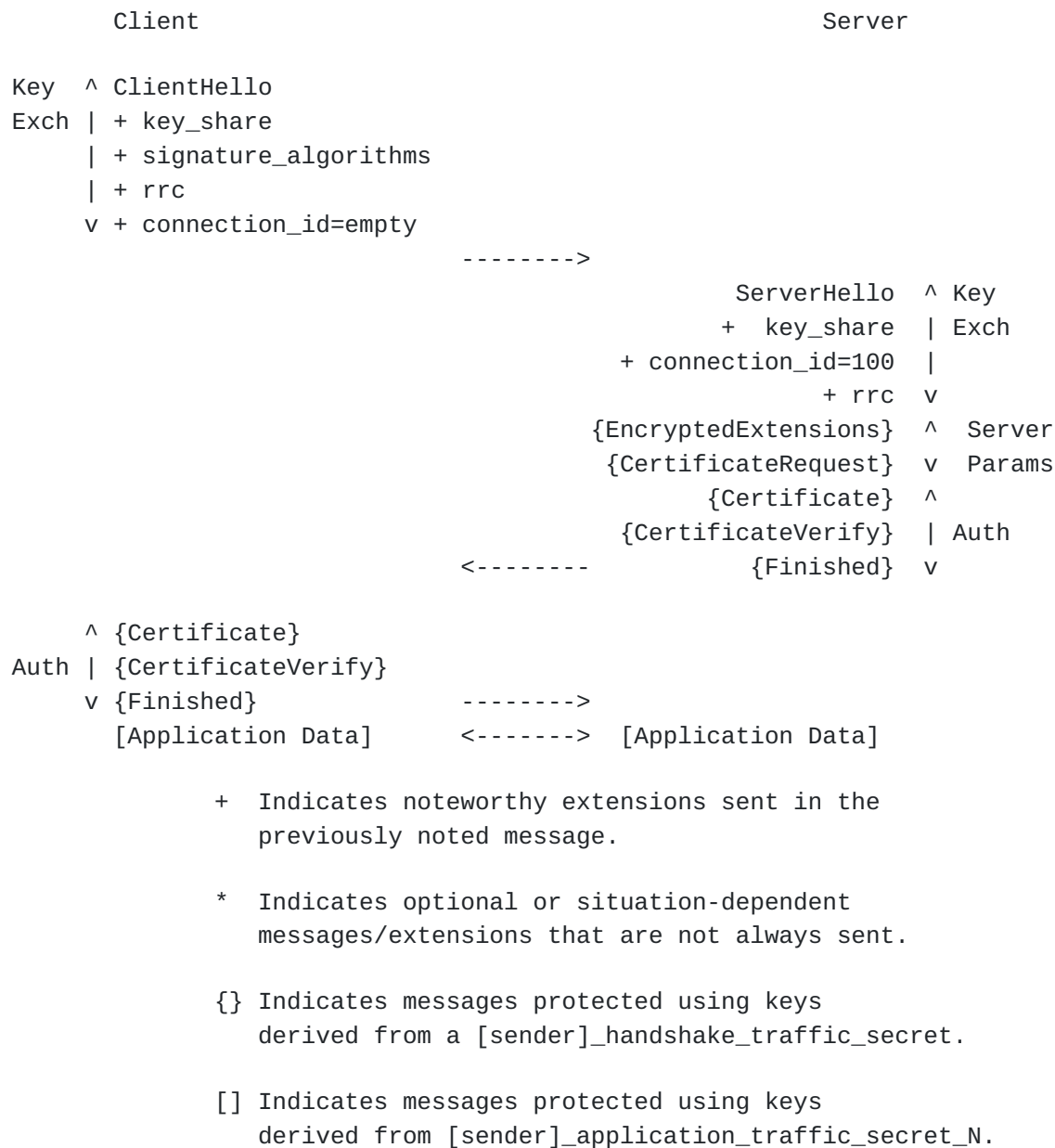
Figure 7: Message Flow for Full TLS Handshake
