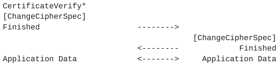
Fig. 1 - Message flow for a full handshake
