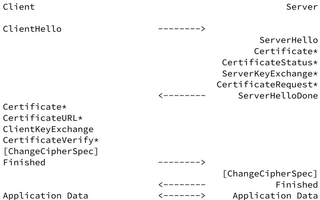
Fig. 1 - Message flow for a full handshake
