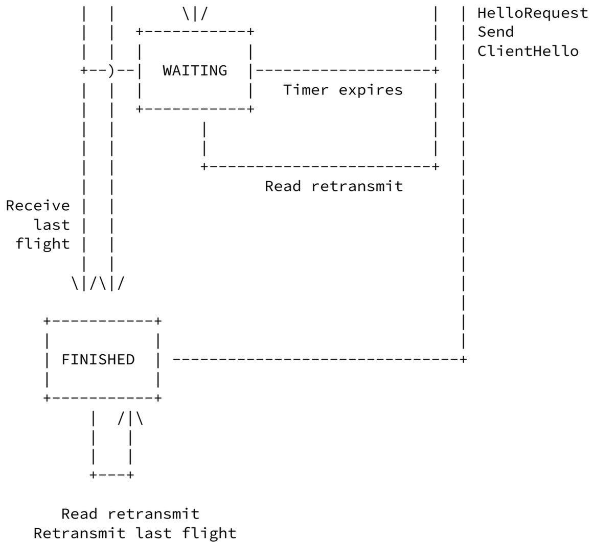
Figure 3. DTLS timeout and retransmission state machine
