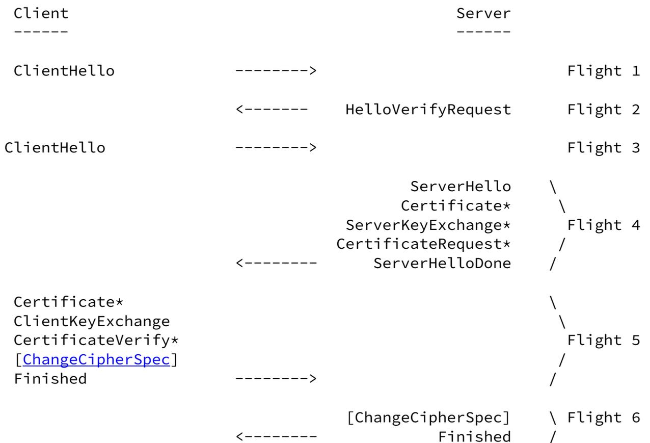
Figure 1. Message flights for full handshake
