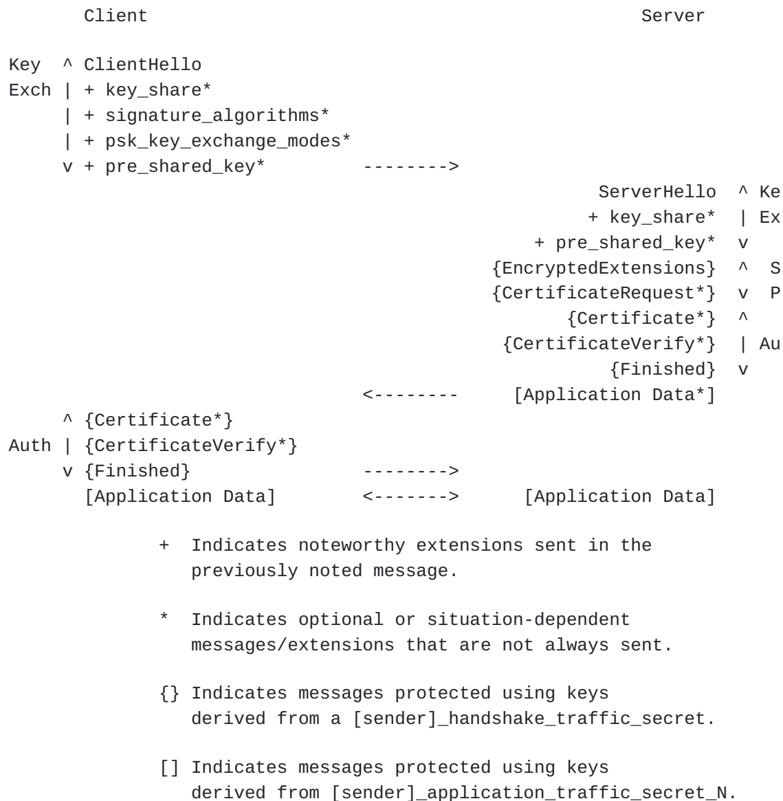
Figure 1: Message Flow for Full TLS Handshake
