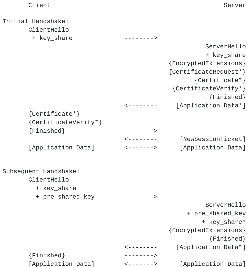
Figure 3: Message flow for resumption and PSK
