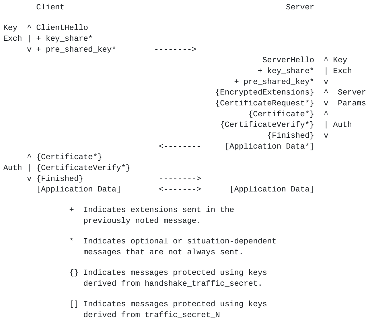
Figure 1: Message flow for full TLS Handshake
