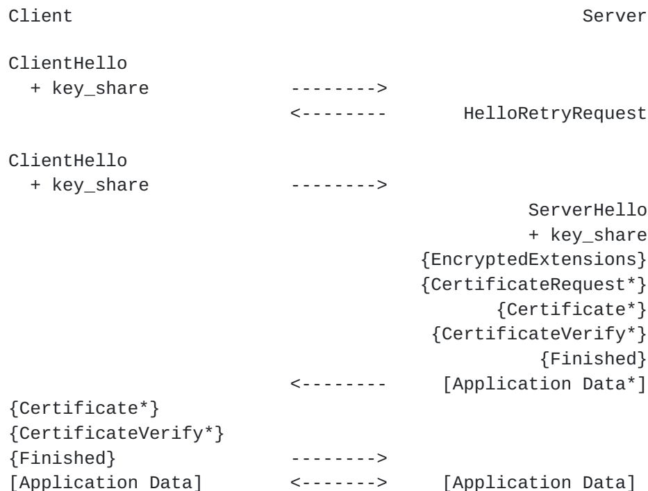
Figure 2: Message flow for a full handshake with mismatched parameters
