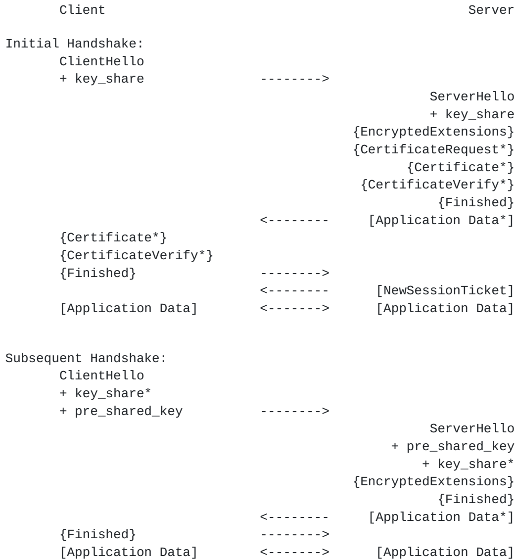
Figure 3: Message flow for resumption and PSK
