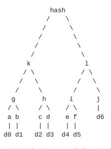
The inclusion proof for d0 is [b, h, 1]. The inclusion proof for d3 is [c, g, 1]. The inclusion proof for d4 is [f, j, k]. The inclusion proof for d6 is [i, k].
