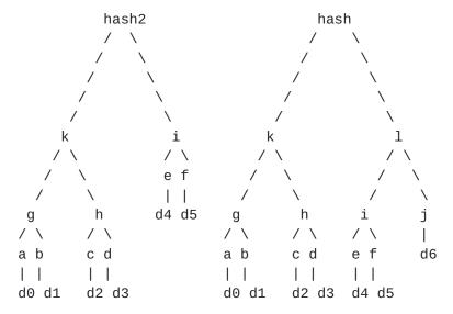
The consistency proof between hash0 and hash is PROOF(3, D[7]) = [c, d, g, 1]. c, g are used to verify hash0, and d, 1 are additionally used to show hash is consistent with hash0.
