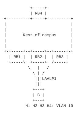
Figure 3.1: An example topology for TRILL Active-Active Edge
