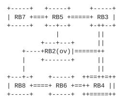
Since RB2 is overloaded it does not know what the distribution tree or trees are for the network. Thus there is no way it can provide normal TRILL Data encapsulation for multi-destination native frames. So RB2 tunnels the frame to a neighbor that is not overloaded if it has such a neighbor that has signaled it is willing to offer this service. RBridges indicate this in their Hellos as described below. This service is called OOMF (Overloaded Origination of Multidestination Frame) service.
