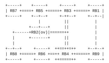
Since RB2 is overloaded it does not know what the distribution tree or trees are for the network. Thus there is no way it can provide normal TRILL Data encapsulation for multi-destination native frames. So RB2 tunnels the frame to a neighbor that is not overloaded if it has such a neighbor that has signaled it is willing to offer this service. RBridges indicate this in their Hellos as described below. This service is called OOMF (Overloaded Origination of Multidestination Frame) service.
