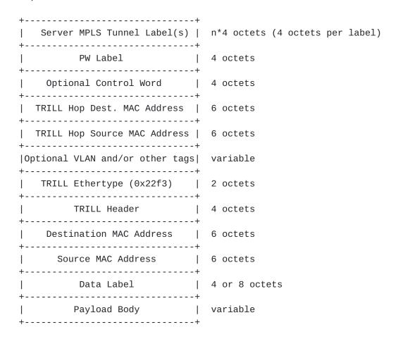
Figure 3. TRILL Data Packet in Ethernet Pseudowire
