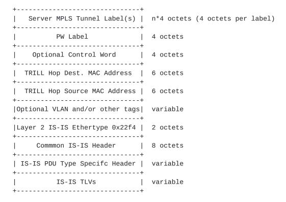
Figure 4. TRILL IS-IS Packet in Ethernet Pseudowire
