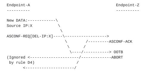
For this case, during the deletion of an IP address, an Abort MUST be ignored if the destination address of the Abort message is that of a destination being deleted.
