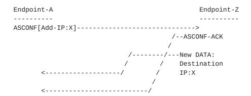
In the above example we see a new IP address (X) being added to the Endpoint-A. However due to packet re-ordering in the network a new DATA chunk is sent and arrives at Endpoint-A before the ASCONF-ACK confirming the add of the address to the association.
