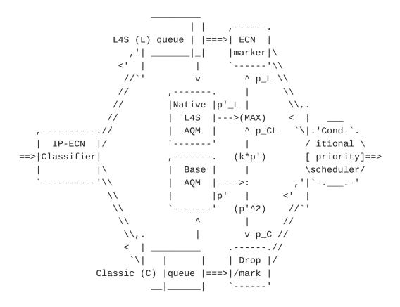
Figure 1: DualQ Coupled AQM Schematic
