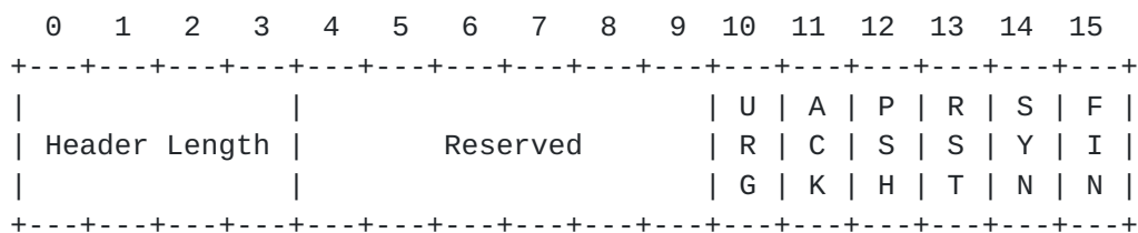
Figure 3: The old definition of bytes 13 and 14 of the TCP header.
