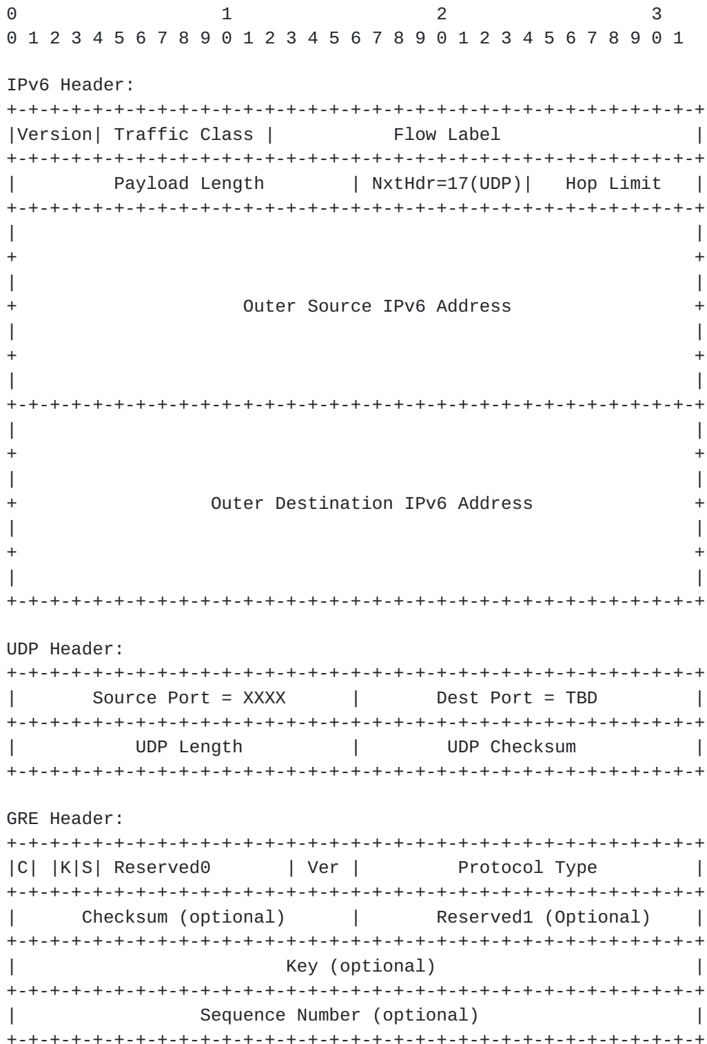
Figure 2 UDP+GRE Headers in IPv6
