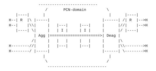
Н = Host requesting end-to-end RSVP reservations R = RSVP router Agg = Aggregator (PCN-ingress-node) Deag = Deaggregator (PCN-egress-node) I = Interior Router (PCN-interior-node)
