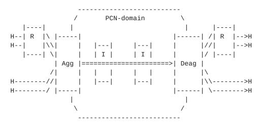
= Host requesting end-to-end RSVP reservations Н = RSVP router R Agg = Aggregator (PCN-ingress-node) Deag = Deaggregator (PCN-egress-node) = Interior Router (PCN-interior-node) I
