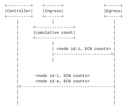
(b) Centralized model feedback procedure
