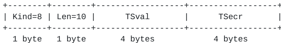
Figure 16 UDP TIME option format
