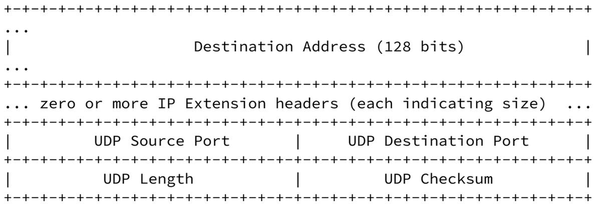
Figure 2 IPv6 datagram with UDP transport payload
