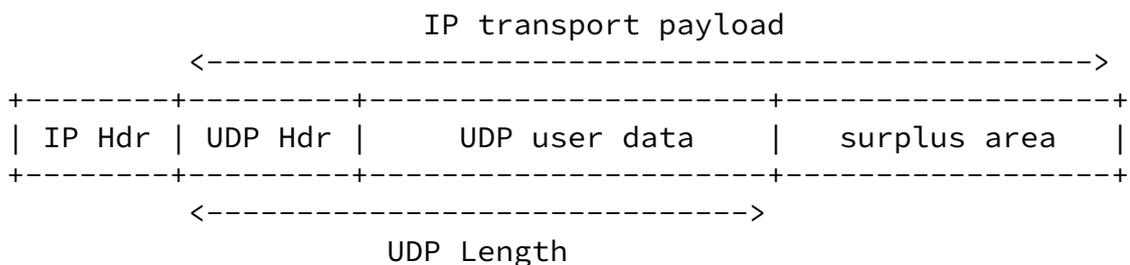
Figure 3 IP transport payload vs. UDP Length
