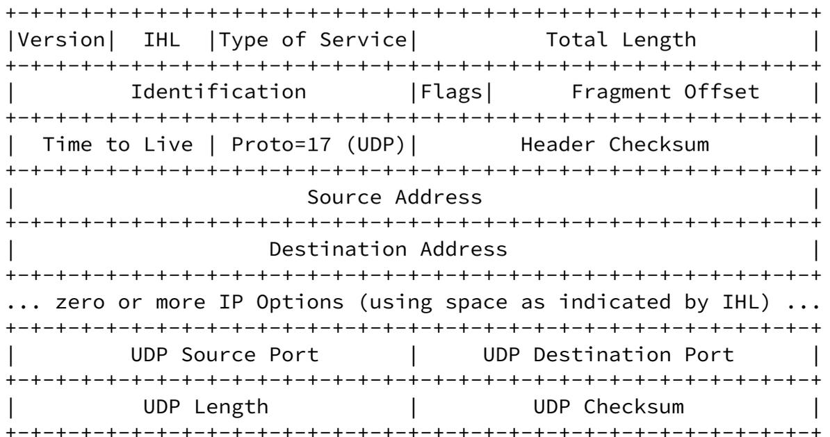
Figure 1 IPv4 datagram with UDP transport payload
