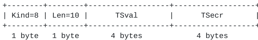
Figure 15 UDP TIME option format
