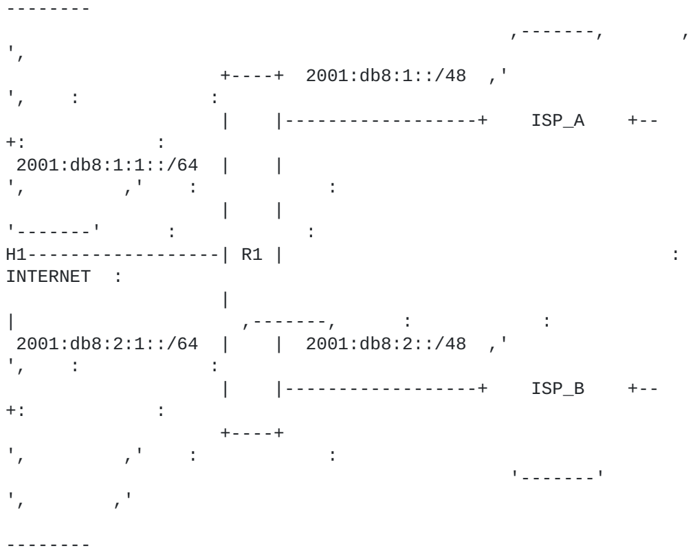
Figure 1: Single Router, Primary/Backup Uplinks
