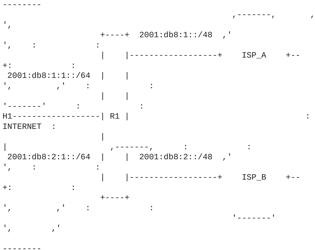
Figure 1: Single Router, Primary/Backup Uplinks
