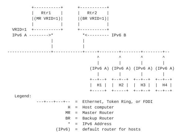
Eliminating all mention of VRRP (VRID=1) from the figure above leaves it as a typical IPv6 deployment. Each router has a link-local IPv6 address on the LAN interface (Rtr1 is assigned IPv6 Link-Local A and Rtr2 is assigned IPv6 Link-Local B), and each host learns a default route from Router Advertisements through one of the routers (in this
