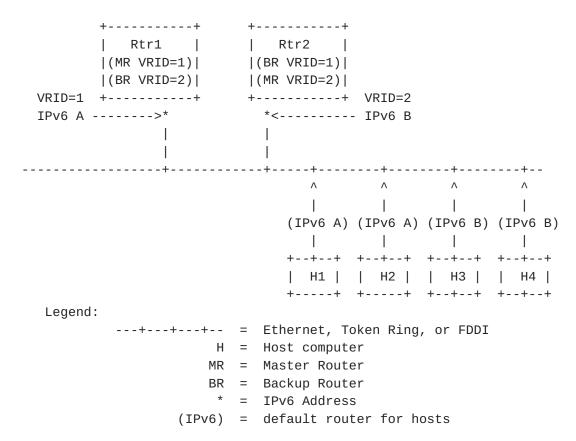
In the example above, half of the hosts have learned a default route through Rtr1's IPv6 A and half are using Rtr2's IPv6 B. The
