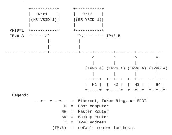
Eliminating all mention of VRRP (VRID=1) from the figure above leaves it as a typical IPv6 deployment. Each router has a link-local IPv6 address on the LAN interface (Rtr1 is assigned IPv6 Link-Local A and Rtr2 is assigned IPv6 Link-Local B), and each host learns a default route from Router Advertisements through one of the routers (in this example they all use Rtr1's IPv6 Link-Local A).
