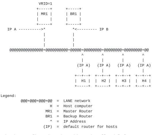
In the above configuration, the end-hosts install a default route to virtual router #1's IP Address (IP A). All the end-hosts (H1-H4) bind (IP A) with the virtual router's (VRID=1) virtual MAC address
