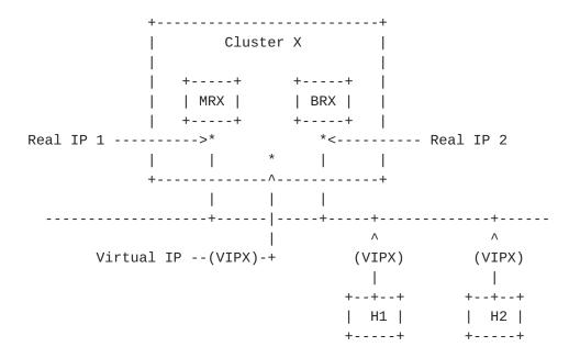
The above configuration shows the most likely utilization of the VRRP protocol. In this configuration, the hosts simply point their default routes at the virtual IP address X (VIPX), and the routers run VRRP
