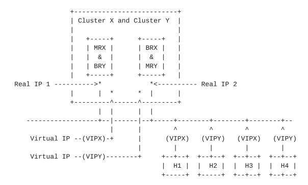
In the above configuration, half of the hosts point their default gateway at cluster X's virtual IP address (VIPX), and half the hosts point their default gateway at cluster Y's virtual IP address (VIPY). This has the effect of load balancing the outgoing traffic, while also providing full redundancy.
