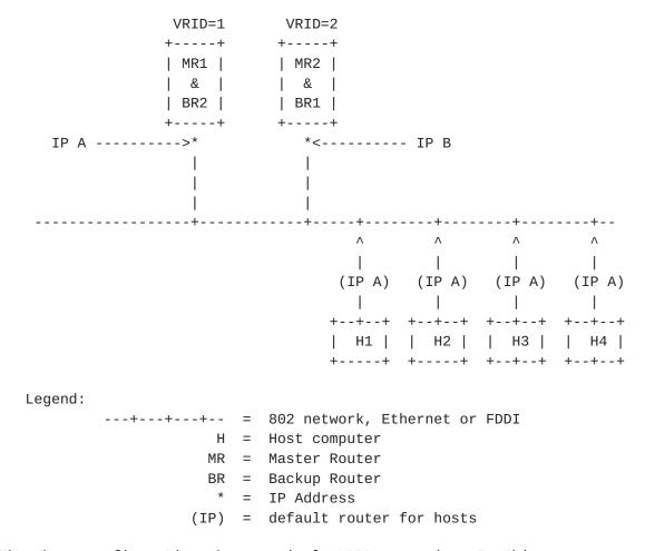
The above configuration shows a simple VRRP scenario. In this configuration, the end-hosts install a default route to the IP address of virtual router #1 (IP A) and the routers run VRRP. The router on the left becomes the Master for virtual router #1 (VRID=1) and the router on the right becomes the Master for virtual router # 2
