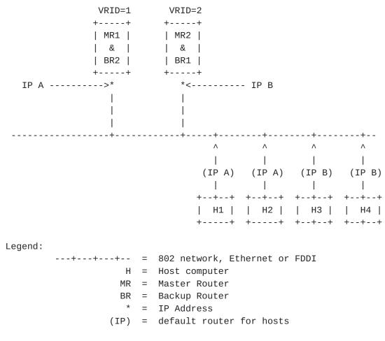
In the above configuration, half of the hosts install a default route to virtual router #1's IP address (IP A), and the other half of the hosts install a default route to virtual router #2's IP address (IP B). This has the effect of load balancing the outgoing traffic, while also providing full redundancy.
