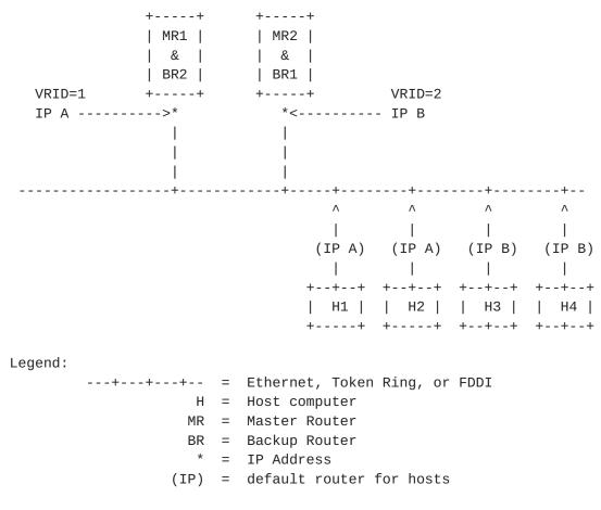
In the above configuration, half of the hosts install a default route to virtual router #1's IP address (IP A), and the other half of the hosts install a default route to virtual router #2's IP address (IP
