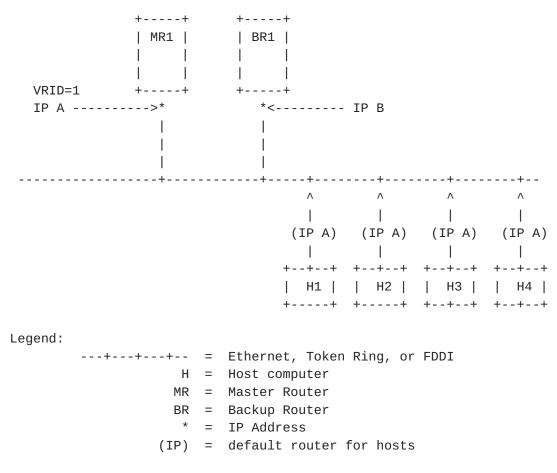
The above configuration shows a very simple VRRP scenario. In this configuration, the end-hosts install a default route to the IP
