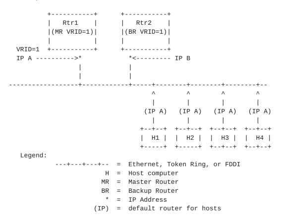
Eliminating all mention of VRRP (VRID=1) from the figure above leaves it as a typical IP deployment. Each router is permanently assigned an IP address on the LAN interface (Rtr1 is assigned IP A and Rtr2 is assigned IP B), and each host installs a static default route through one of the routers (in this example they all use Rtr1's IP A).
