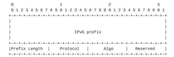
Algo field MUST be set to 0 if the default algorithm is used. Algo field is set to 1 if Strict Shortest Path First (Strict-SPF) algorithm is used. For Flex-Algo, the Algo field MUST be set with the algorithm value (values can be 128-255).
