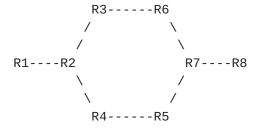
Figure above, which is a simplification of the diagram used in [RFC8287] illustrates this point through an example. Node Segment IDs for R1, R2, R3, R4, R5, R6, R7, and R8 for the default algorithm are 5001, 5002, 5003, 5004, 5005, 5006, 5007, and 5008, respectively. Nodes R1, R2, R4, R5, R7, and R8 also participate in Flexible Algorithm 128. Their corresponding Node Segment IDs for the algorithm are 5801, 5802, 5804, 5805, 5807, and 5808, respectively.
