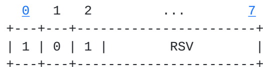
Figure 25: Dispatch format for uncompressed CCNx Content objects
