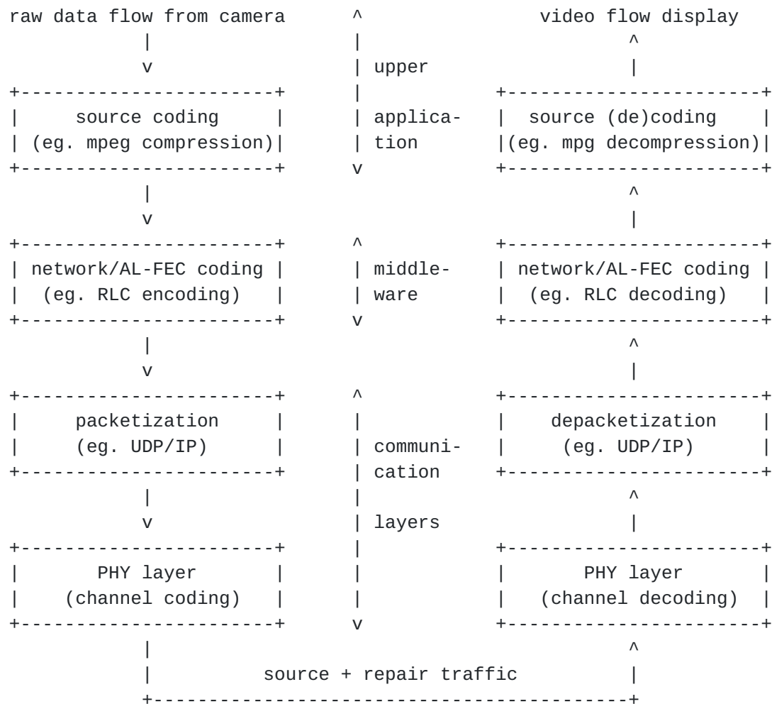
Figure 2: Example of end-to-end flow manipulation with Network Coding between the application and UDP layers (as with RMT or FECFRAME architectures). Other architectures are possible, for instance with network coding below the transport layer in order to allow re-coding within the network.
