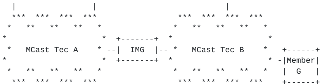
Figure 2: Reference scenarios for hybrid multicast, interconnecting group members from isolated homogeneous and heterogeneous domains.
