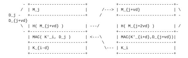
Figure 4: Immediate authentication packet example.  $D_j = H(M_{j+vd})$  $| M_j \text{ and } D_{j+vd} = H(M_{j+2vd}) | M_{j+vd}.$
