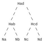
Figure 9: Hash tree over receiver nonces. Node  $H_{ab} = H(N_a, N_b)$ .  $H_{ad} = H(H_{ab}, H_{cd})$ .
