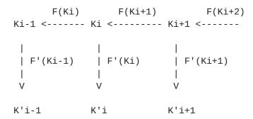
Figure 1: TESLA key chain and the derived MAC keys
